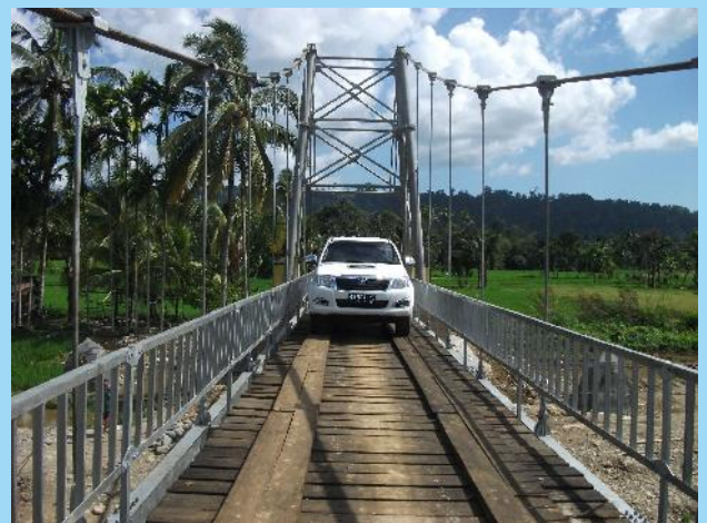
Loading Test / Uji Coba
